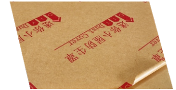
Take out the plexiglass and tear off the kraft paper with text on each piece of plexiglass
