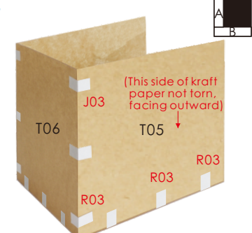
The junction of two pieces of plexiglass needs to be fixed with R03 (to prevent the plexiglass falling off)
